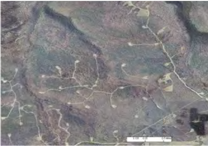
Infrastructure including roads, well pads, and pipelines are part of natural gas development. Maintenance of these features results in herbaceous edges. Note the predominantly forested landscape.
